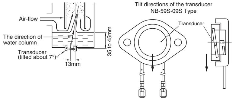
The arrows indicate the tilt direction of the transducer.
