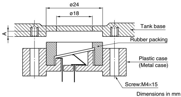
The transducer can break off if the A dimension depth is shallow. TDK recommends a 2mm A-dimension depth and a screw tightening torque of 0.6N•m.
